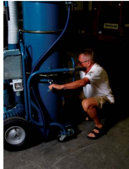
The container is attached to the machine by two fasteners.
