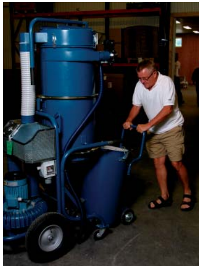
When emptying the container, it is unclipped and removed away from the machine. After that has been done the sack can be taken out of the container.
